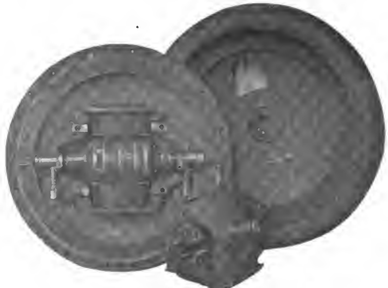
WHEEL DISSEMBLED, SHOWING MOTOR FIELDS AND ARMATURE.
